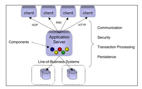
Figure 1. Application Server Architecture
